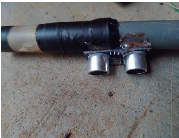
Fig. 6: The Ultrasonic sensor used in the detection of an obstacle
