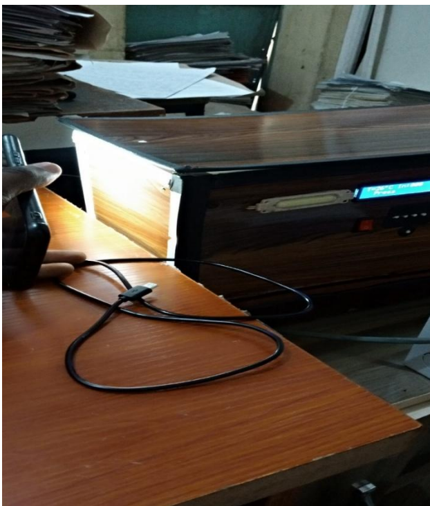
Fig. 17. The outside LDR that is used to control the front light of the house will go off during day light. That is, if the research is exposed to light, the front light will not come on until it sees dark the LDR
