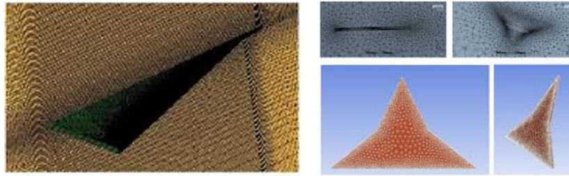
Fig. 8: Hybrid computational mesh used for aerodynamic simulation.
