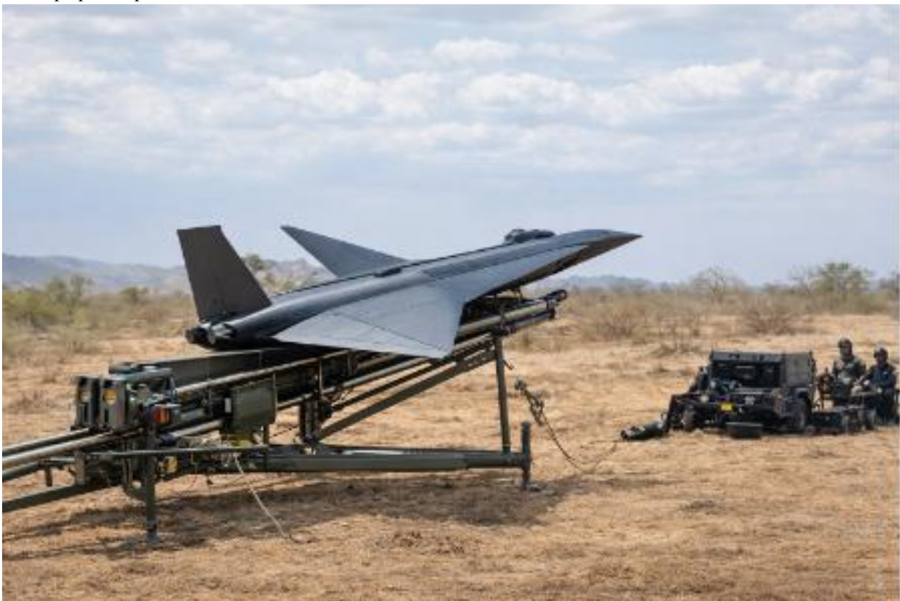
Fig. 7: Field deployment configuration of HATSABIBI-26A Delta-Wing UAV on portable rail launcher.
