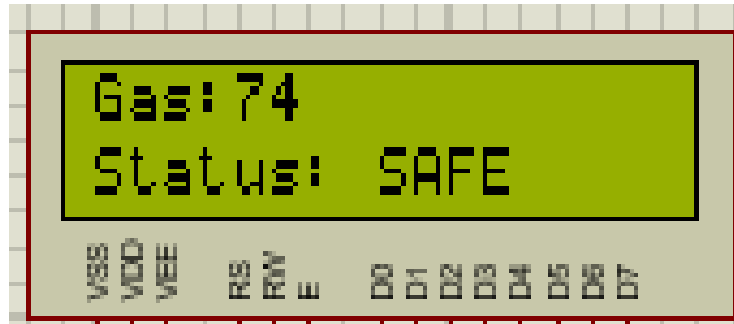
Figure 5.8: The Simulation Result Display there is no Gas Leakage.
